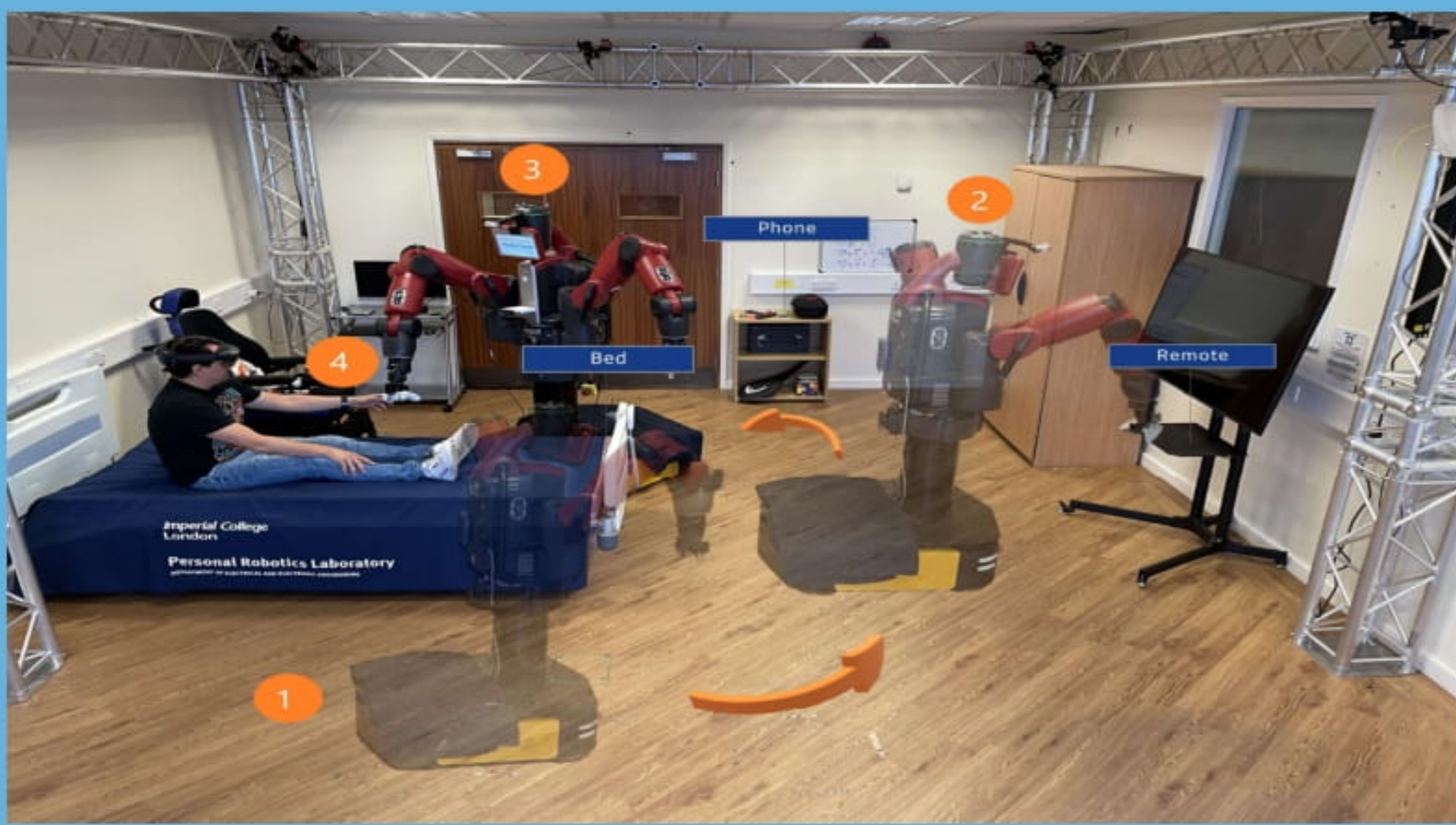
Figure 1. Current affordance-based AR HMD UIs for robot control would require at least four input commands to complete a task such as "Pick-up the remote and put it on the bed": 1) [Robot's starting position] approach the tv-stand, 2) pick-up the remote, 3) approach the bed and 4) give the remote. 1
